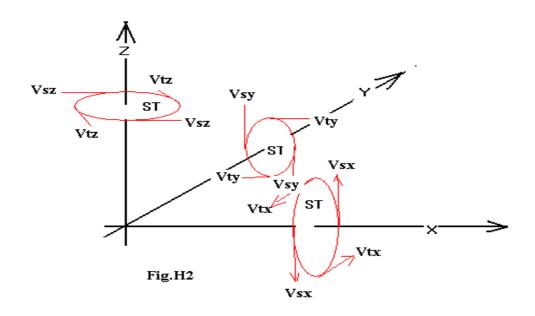
$$V_{S_{XYZ}} = \sqrt{(\pm V_{S_X})^2 + (\pm V_{S_Y})^2 + (\pm V_{S_Z})^2}$$
